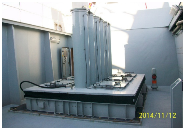
Weapon/Payload Modules (StanFlex Modular VLS, Photo by AOC)
